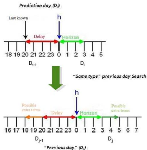
Figure 3 Demand prediction algorithm diagram
